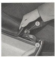
Place cover F on the folded top well by fitting rear eyelets D on hooks E (page 14) then catches G in detents  $\mathbf{H}$ , spring hooks  $\mathbf{I}$  in holes  $\mathbf{L}$  and snap on the button fasteners  $\mathbf{M}$ .
