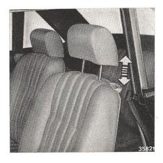
For access to the rear compartment push down lever **C** and tilt backrest downward.
